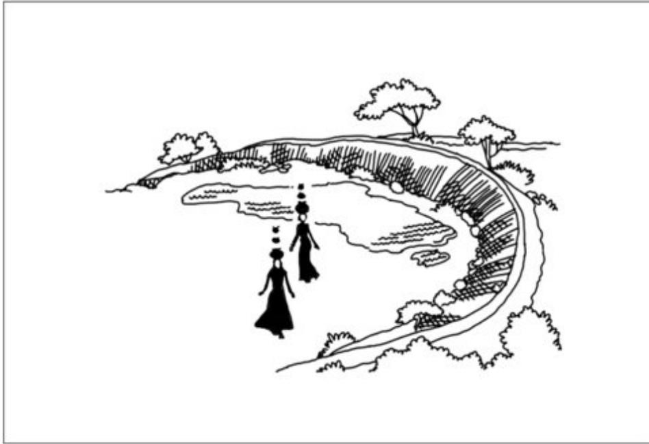
**Johad** is the name given to small earthen check dams. Due to the extreme heat and desert conditions in Rajasthan, rainwater is harvested in these tanks. Johads are formed when semi-circular mud barriers are built across slopes to catch the monsoon run-off. The rainwater is harvested in these tanks and held for agriculture.
